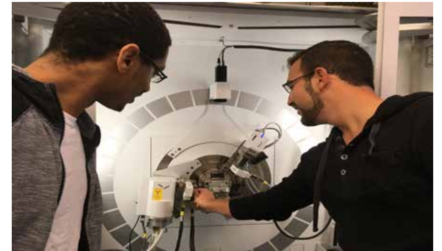
MSE students, Jesse Johnson (senior) and John Salasin (graduate), both use the Panalytical Empyrean X-ray powder diffractometer that is part of the JIAM X-Ray Diffraction Core Facility for their research.
